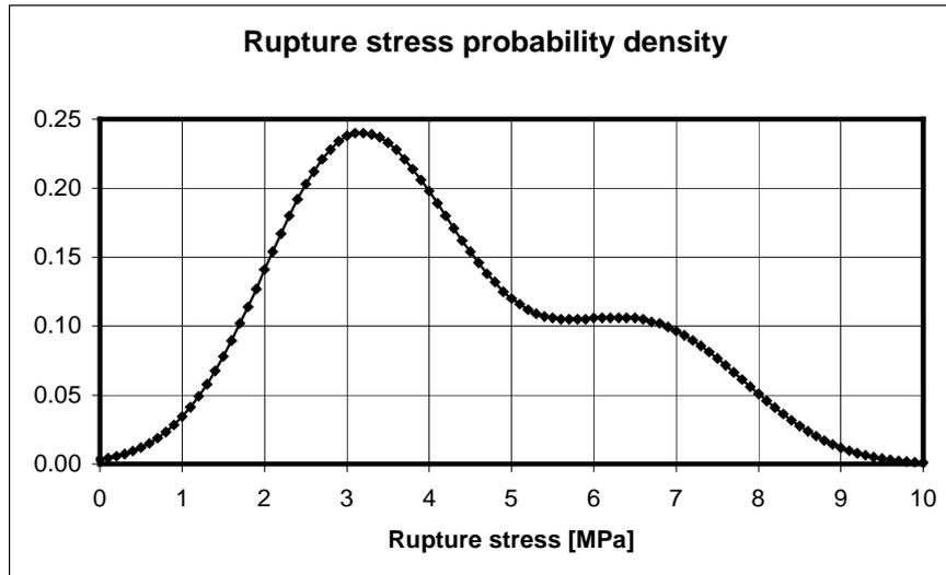
Figure 1 : Rupture stress probability density obtained with a kernel estimation of density from the results of the laboratory tests
