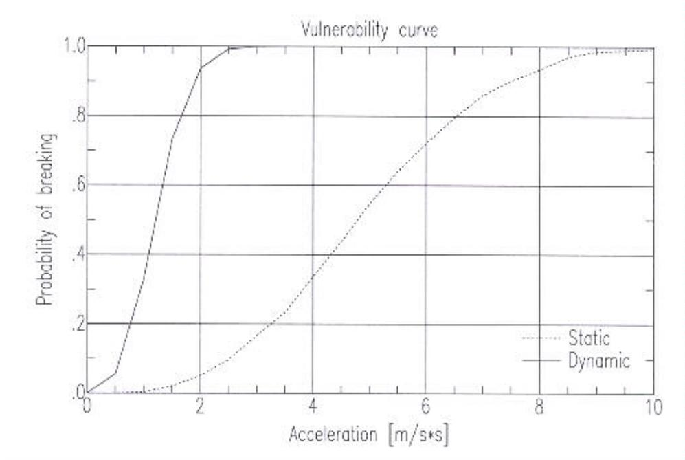
Figure 3 : Vulnerability curves for a test stalactite (L about 80 cm and average D of 2 cm), under the hypothesis of a rigid body (dashed line) or accounting for full dynamic amplification of the motion (solid line)
